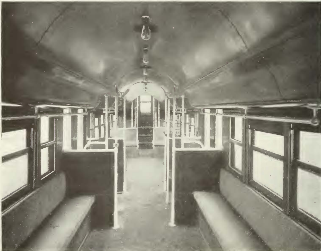
DOUBLE-DECK CAR FOR COLUMBUS Stairway arrangement occupies a minimum of seating space
