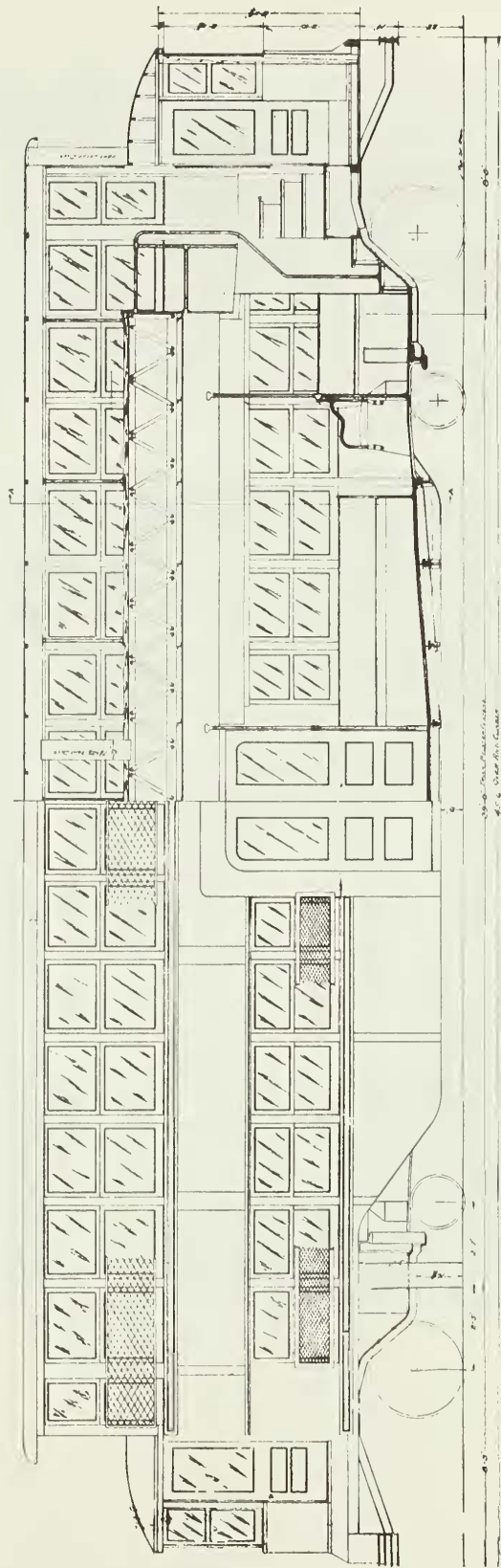
DOUBLE-DECK CAR FOR COLUMBUS. Track to side sill 8 in.; side sill to trolley board, 12 ft. 5 in. Track to step, 11 ft. 3/8 in. Weight of body, less electrical equipment, but including air-brake equipment, 31,640 lb. Seating capacity, lower deck, 45; upper deck, 40
